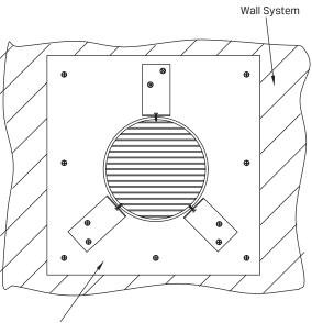
16mm Fire Resistant Grade Plasterboard support pad 100mm larger all around than aperture fixed with 40mm x 10G laminating screws to face of the wall at approximately 250mm centres and sealed along the perimeter with 6mm fillet of Kilargo Intumescent Mastic.
