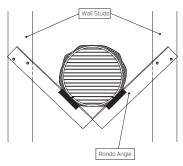
Guard Removed for clarity FACE FIXING Alternative fixing method Kilargo Intumescent
