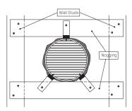
Guard Removed for clarity FACE FIXING Alternative fixing method Kilargo Intumescent fire damper supported by studs noggins
