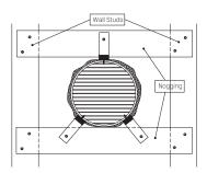
Guard Removed for clarity FACE FIXING Alternative fixing method Kilargo Intumescent fire damper supported by studs noggins
