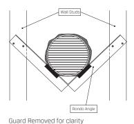
FACE FIXING Alternative fixing method Kilargo Intumescent fire damper supported by external Rondo angle hung between studs
