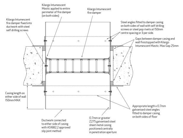
Insulation value of the damper negates the need for additional insulation cladding, as per ASI668.1 Note C3.4
