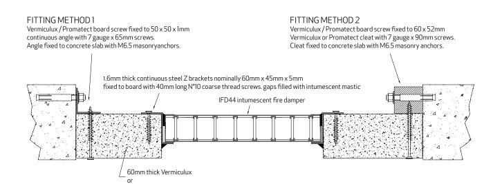
Note: This system is NON-LOADBEARING and if used in a trafficable area appropriate signage and were necesarry a load bearing grate should be utilised to minimise the risk of injury arising from persons walking upon it.
