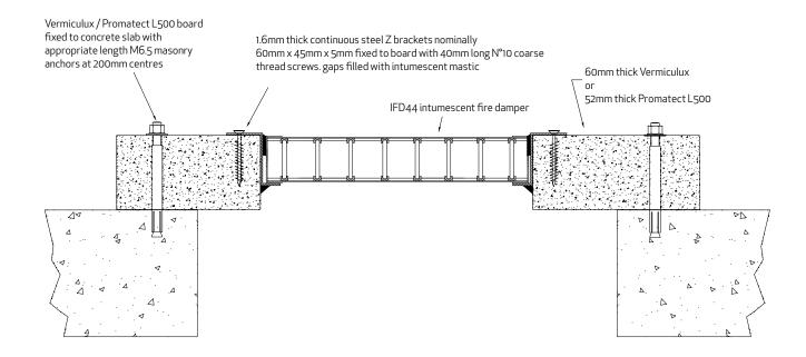
Note: This system is NON-LOADBEARING and if used in a trafficable area appropriate signage and were necesarry a load bearing grate should be utilised to minimise the risk of injury arising from persons walking upon it.
