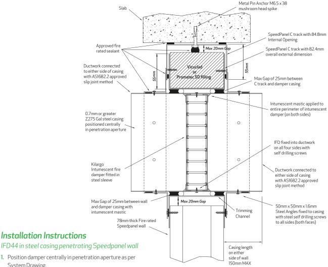
IFD44 in steel casing penetrating Speedpanel wall
